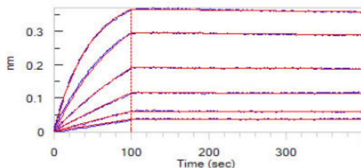
Loaded Mouse / Human chimeric FMC63 MAb (human IgG1) on AHC Biosensor, can bind Human CD19 (20-291), Mouse IgG2a Fc Tag (Cat. No. CD9-H5258) with an affinity constant of 0.487 nM as determined in BLI assay (ForteBio Octet Red96e) (Routinely tested).
