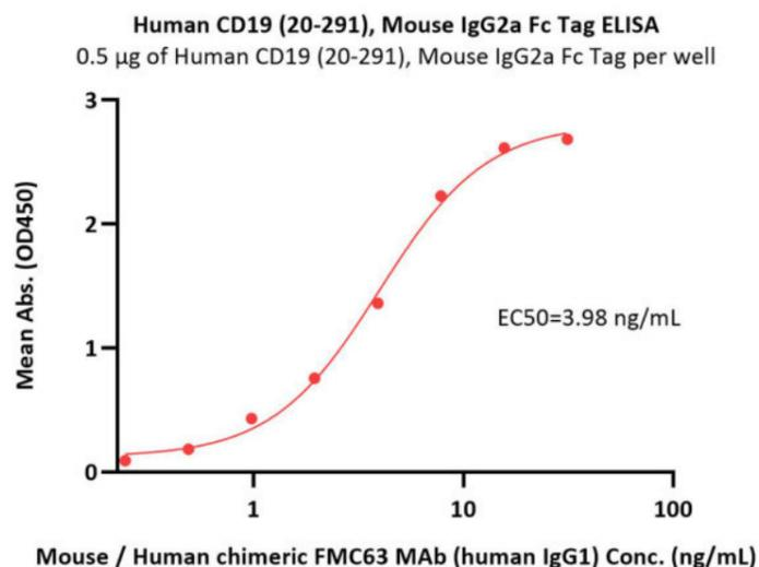
Immobilized Human CD19 (20-291), Mouse IgG2a Fc Tag (Cat. No. CD9-H5258) at 5 µg/mL (100 µL/well) can bind Mouse / Human chimeric FMC63 MAb (human IgG1) with a linear range of 0.5-8 ng/mL (QC tested).
