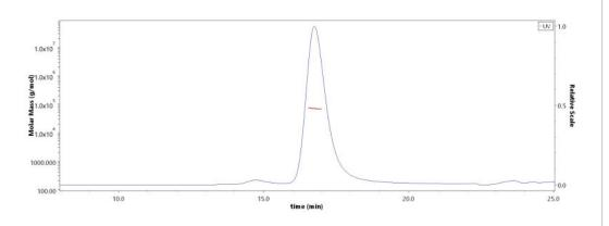
The purity of Biotinylated Human CD1d&B2M Monomer Protein (Cat. No. CDM-H82E9) is more than 90% and the molecular weight of this protein is around 55-75 kDa verified by SEC-MALS.
