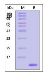
Human NT-3 Protein, Tag Free on SDS-PAGE under reducing (R) condition. The gel was stained with Coomassie Blue. The purity of the protein is greater than 90% (With Star Ribbon Pre-stained Protein Marker).
